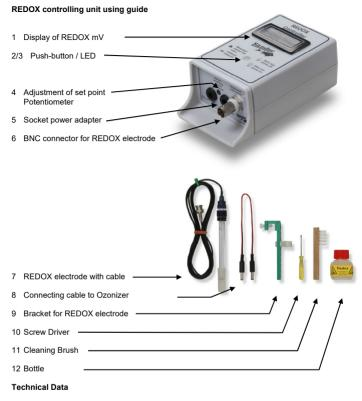
Range of usage: 0 bis 1000 mV Power supply: 12 VDC Current consumption: 100 mA max. Switching capacity: 12 VDC / 4A
