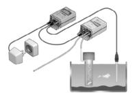
A Sander ozone generator of the product series Certizon or S should be connected using the delivered connecting cable for REDOX (8). The REDOX measuring and regulating unit are delivered with a special power adaptor.
