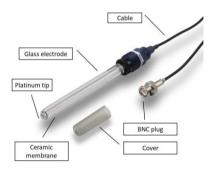
To always get exact measuring amounts and the best results, the maintenance as describe above should be done accordingly and the REDOX Electrode itself may be exchanged yearly.
